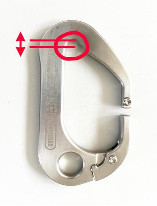
A close-up photograph of a silver metal carabiner. A red circle highlights the area where the gate meets the body of the carabiner. Two red arrows point to this area, one vertically and one horizontally, indicating the location of maximum wear. |
